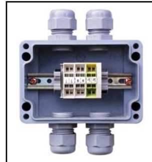
L13X1- junction box – polyester with mini terminals 4 x 2,5 mm 2 , 800V, 24A
