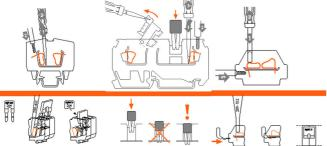
At some types of terminals with cage clamp it is necessary to use a greater one terminal when connecting a wire with a ferrule. E.g. for connection of a 2,5 mm<sup>2</sup> wire with the ferrule, it is necessary to use a terminal block 4,0 mm<sup>2</sup>.
