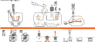
In the case of some types of spring-cage terminal blocks, connecting a wire with a ferrule requires the use of a terminal block with a connection cross-section one grade higher than the wire crosssection. E.g. a 2.5mm2 wire with a ferrule requires the use of a
